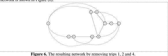
The result of minimum cost flow algorithm in the network of figure (6) is:  $s \to 3 \to 6 \to 5 \to 7 \to t$ . Also the cost of this iteration is 1534. The minimum cost of the algorithm is 947 which is obtained for the values  $B_1 = 1$  and  $B_2 = 2$ . This problem is modeled as an integer programming in AMPL software and solved with this software. The results of AMPL software are as the same as the proposed method.
