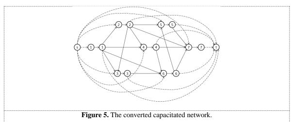
The minimum cost network flow algorithm is used to construct a flow of value 3 in the capacitated network. The result of this algorithm is as follows:
