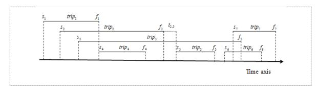
**Figure 1.** An instance of bus scheduling problem with 7 trips.
