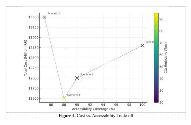
This graph illustrates the natural trade-off between cost and accessibility for all considered deployment scenarios. As shown by the results, higher accessibility (Scenario 4 with full coverage) comes with high costs, while relatively low cost configurations (Scenario 3) trade off part of the access. In addition, since the CO<sub>2</sub> emissions are color-coded, one also sees the environmental trade-
