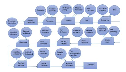
Figure 5. Conceptual model of residential house construction operations
