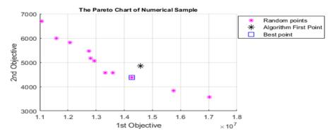
Figure 8. The Pareto Front Chart of Numerical Sample
