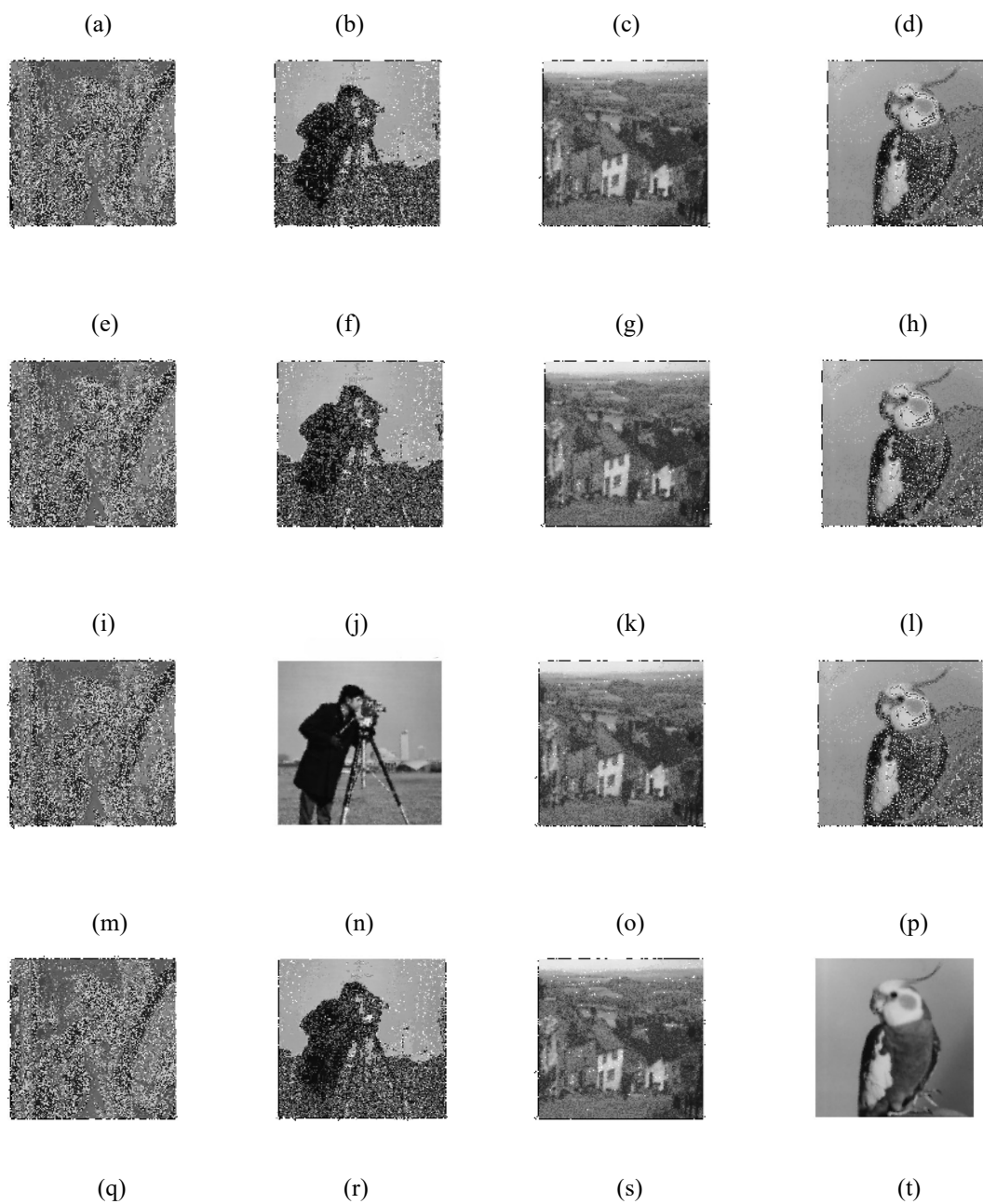
Figure 5: The noisy images corrupted by 75% salt-and-pepper noise: (a)–(d), the restored images via HTTHSLS: (e)–(h), HTTWYL: (i)–(l), HTHP : (m)–(p), and MTTHSLS: (q)–(t)
